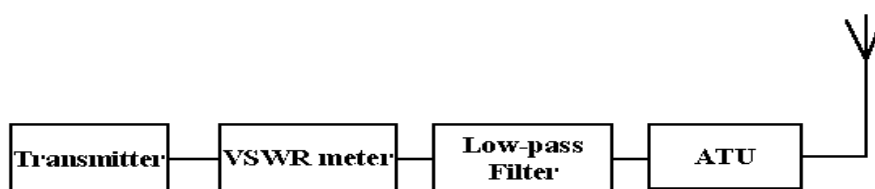
A low-pass filter fitted to a HF transmitter
